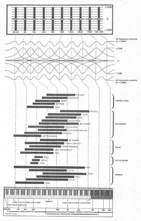
Only the fundamentally generated frequencies are shown. Harmonics are extended both above and below these fundamentals, and are controlled by the EQ bands at the outer ends of the spectrum.
