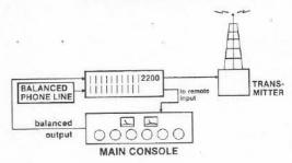
The 2200 Graphic Equalizer is ideally suited for use as a combination telephone line and transmitter equalizer. Telephone lines used for remote broadcasts very frequently are not of the highest quality. Even Class A lines have been known to suffer from frequency response deviations. One 2200 installed in the main control room can take care of the phone line, and equalize the transmitter's signal too.
